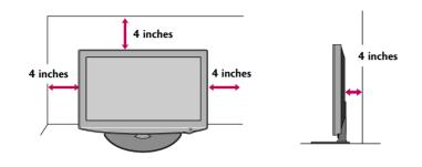
▲ CAUTION ► Ensure adequate ventilation by following the clearance recommendations. ► Do not mount near or above any type of heat source.
